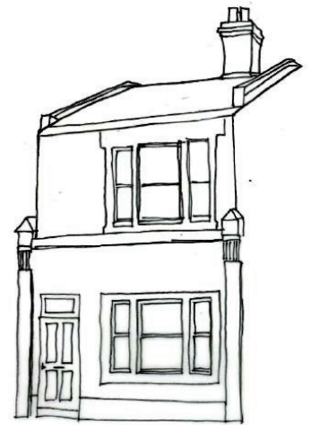
Example of a good conversion; the conversion has retained the shopfront surround but new windows and a door have been inserted which reflects the Victorian style of property.
