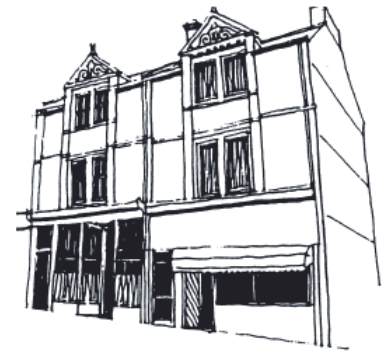
The left hand building has a better scaled fascia
