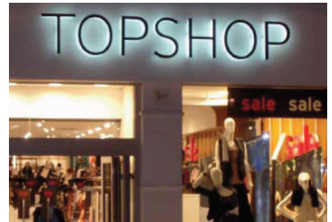
Above example of Halo lighting – letters are raised and lit from behind
