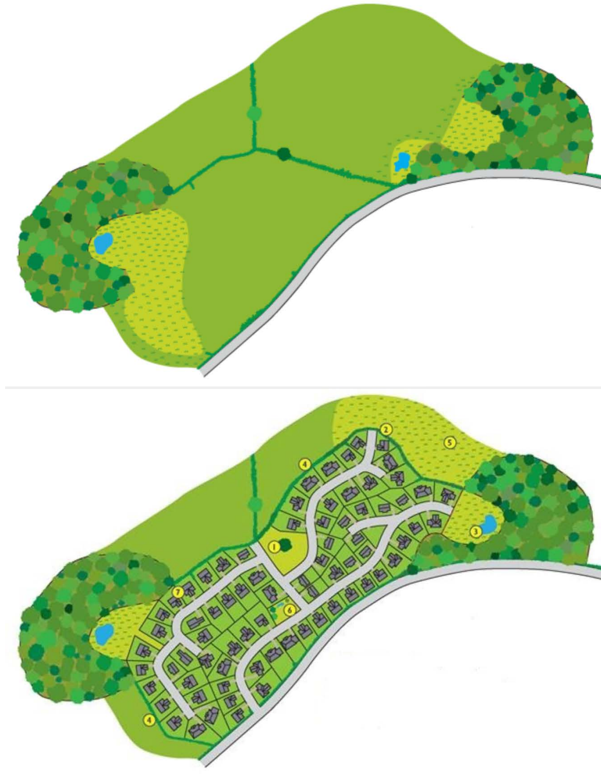
Figure 2: Pre and Post-development: How wildlife features can be avoided, mitigated, compensated, enhanced and managed
