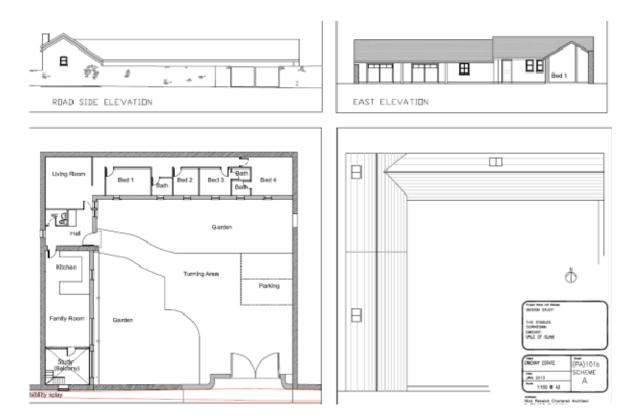
The plans show a single storey building of between 4m and 5m in height, with a stepped roof line. The L shaped footprint is approximately 22m deep by 24m wide with a span of 5m.
