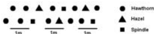
For best results, use hawthorn, hazel and spindle planted in two rows.
