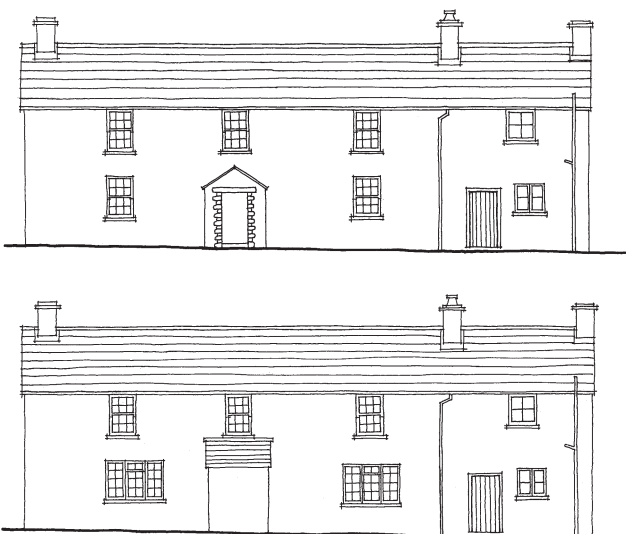
The removal and replacement of original windows can upset the balance of a house
