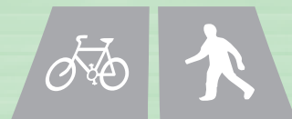
Ground markings indicate segregated route for pedal cycles and pedestrians only (please keep to the correct side)
