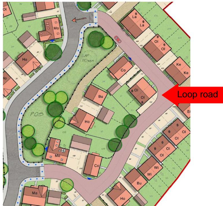
The extract below is from plan 'C/S110-1 rev 9', approved on 8/10/2019, under application 2014/01424/1/CD, in discharge of condition 4-Highway engineering details. It shows where the main estate road with raised footways becomes the shared surface loop road with no raised footway.
