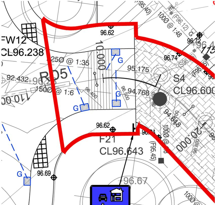
A sign stating that the loop road is a 'shared surface zone' is proposed to be added at each end of the loop road.
