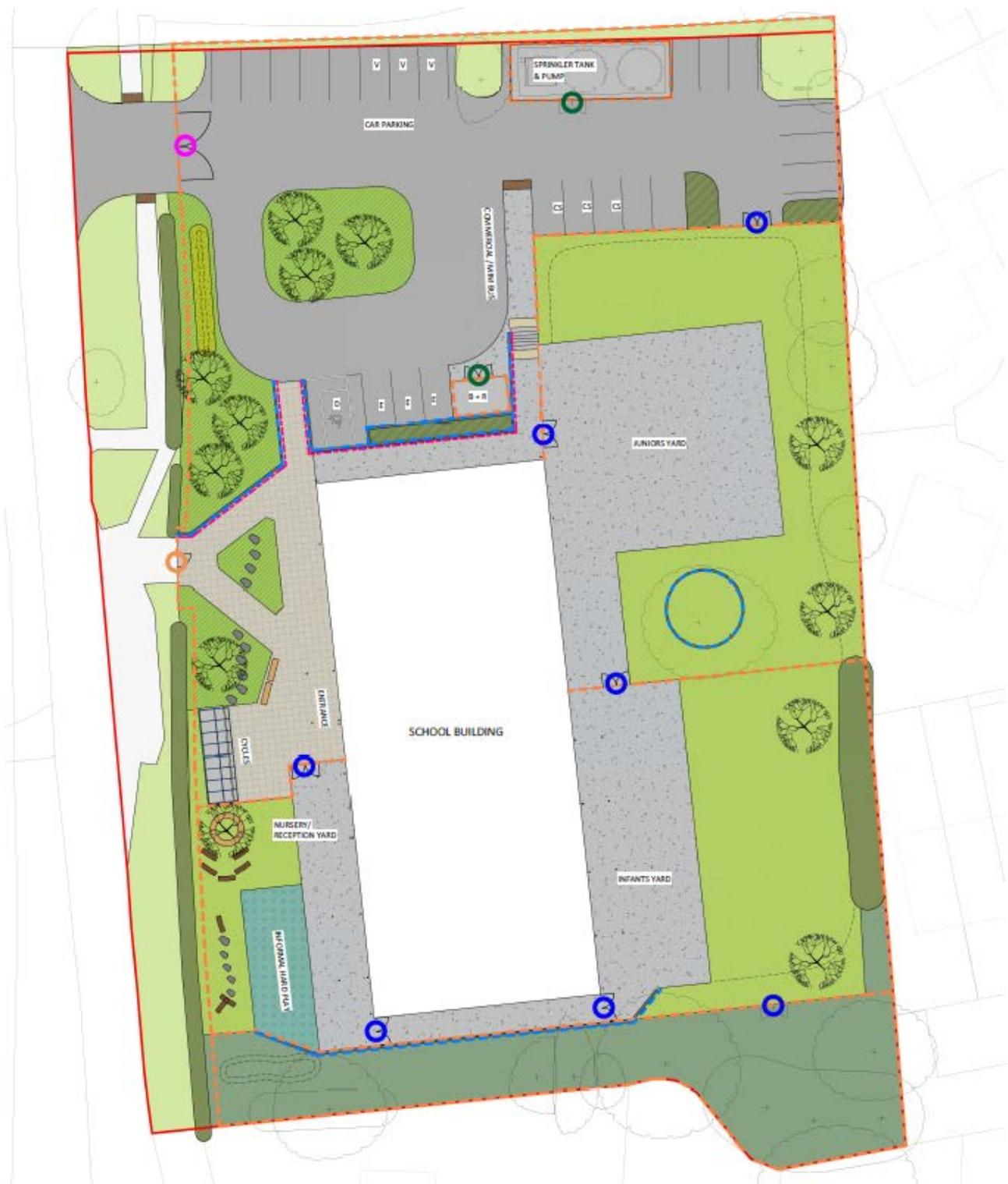
Whereas the existing school building is located closer to the north of the site, with open space to the south, the new school would be located in the southern part of the site, with an enlarged parking and circulation area to the north. The vehicular access would remain in essentially the same place as that which serves the existing school. There would be 24 parking spaces provided, comprising 20 for staff, 3 visitors' spaces and 1 commercial/minibus space.
