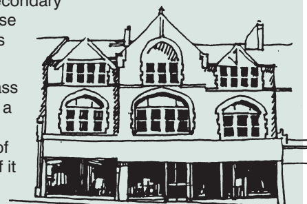
The scale of the fascia disrupts the rhythm of the street
