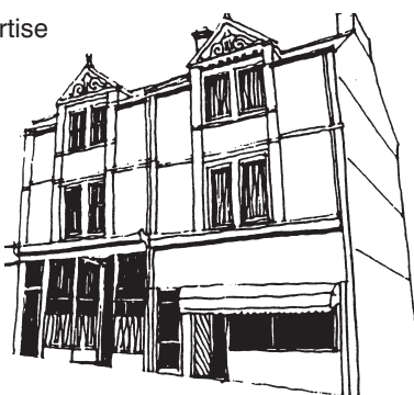
The left hand building has a better proportioned fascia
