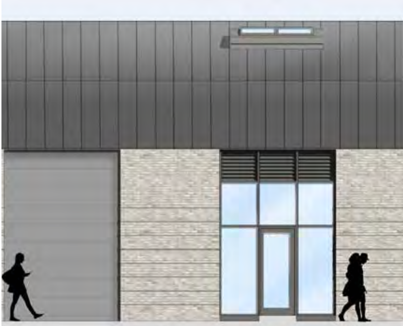
Option 2: metal cladding finish
