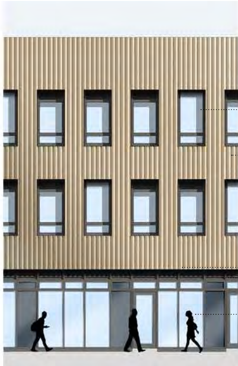
Option 3: Curtain walling with back painted glass at column intervals
