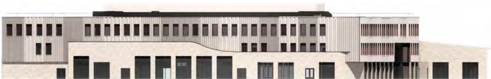
Option 1: Step in Parapet height
