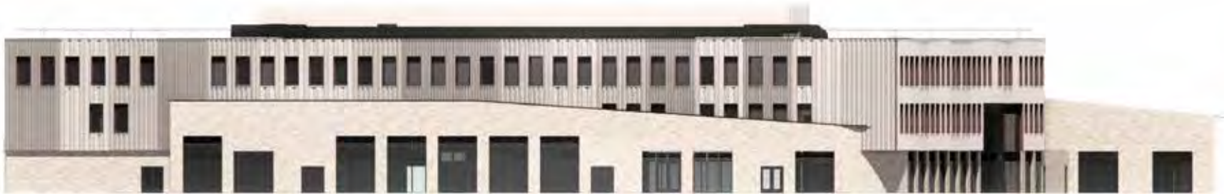
Option 2: Parapet line falls from the end of the double height spaces
