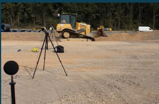
Noise measurement of dozer in action
