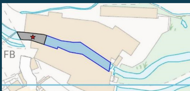
Re-directed River Culm (blue) and 60 m section of retained culvert (grey) housing bat roost location (star).
