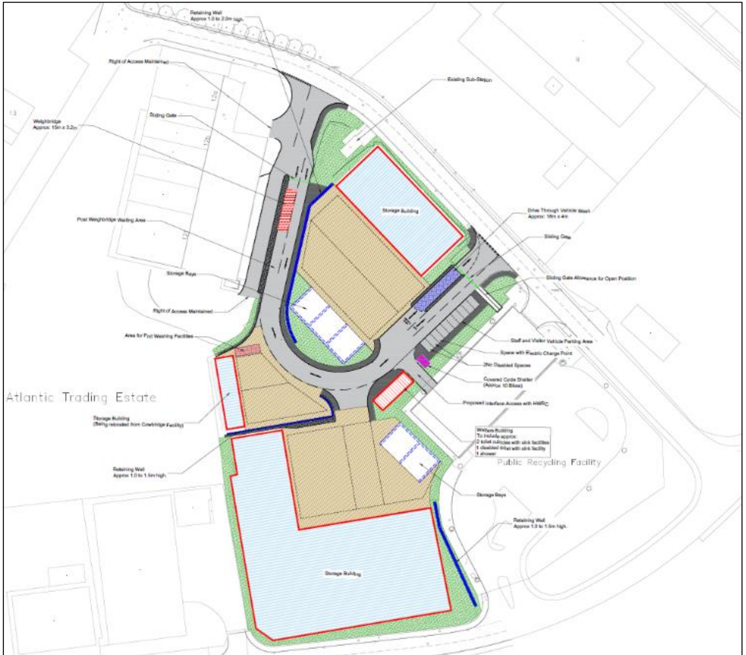
Figure 4: Proposed Site Layout & Access Arrangements
