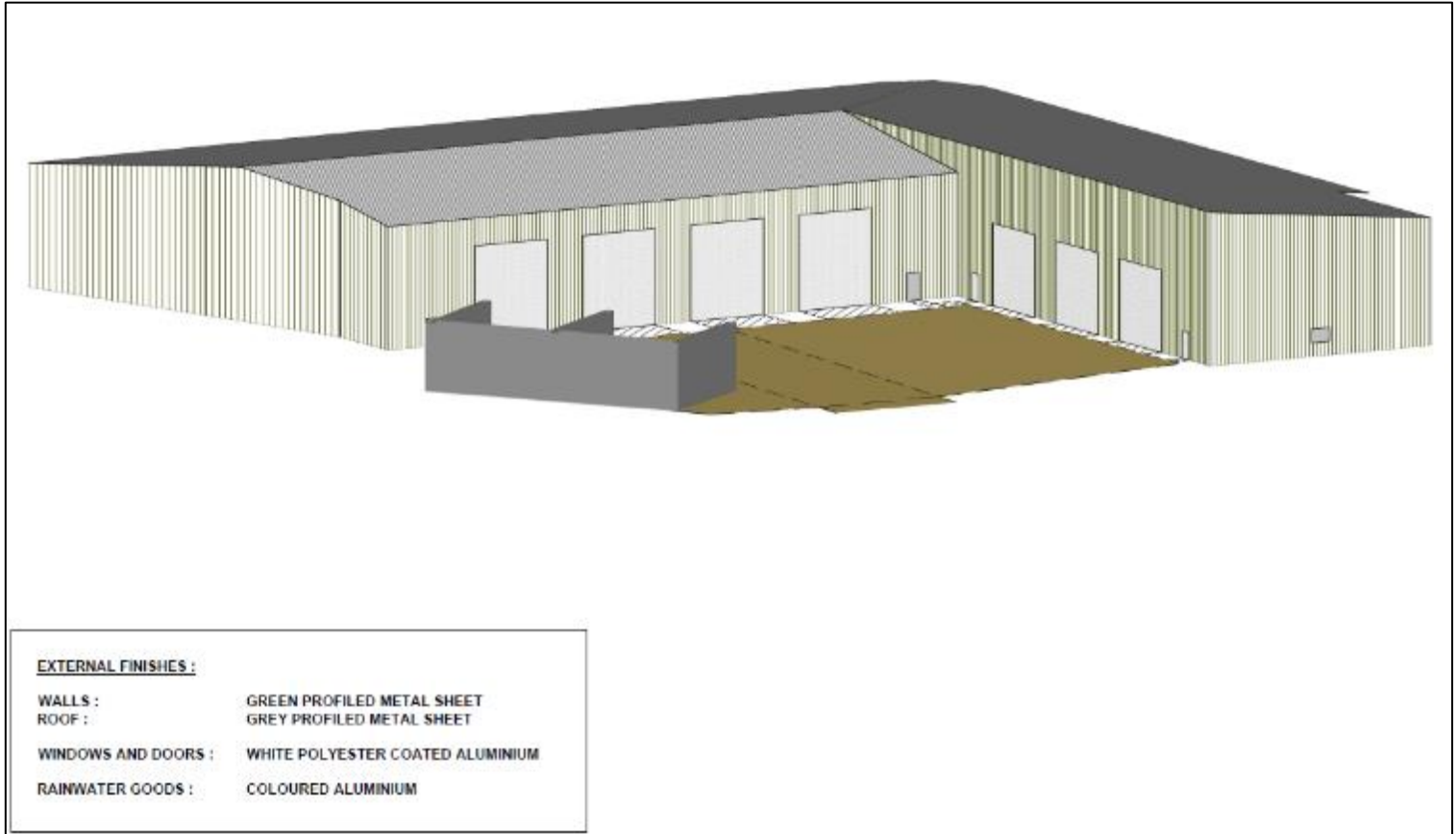
Figure 5: Proposed Main Storage Building Principle Elevation
