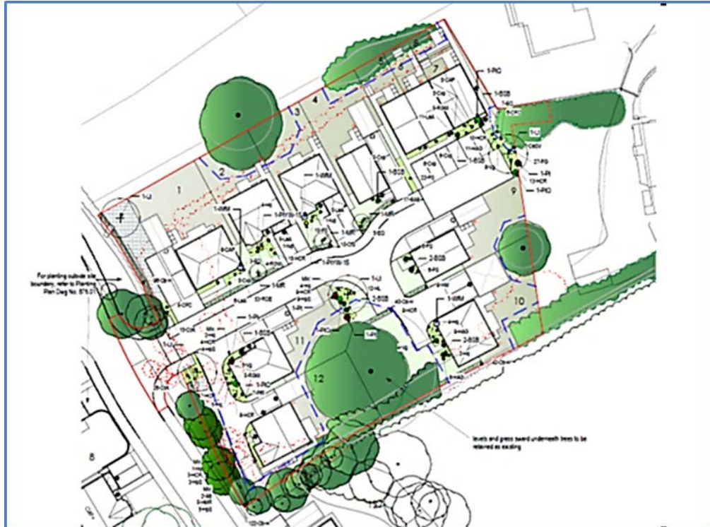
Figure 3: Example of a Tree Protection Plan (TPP)
