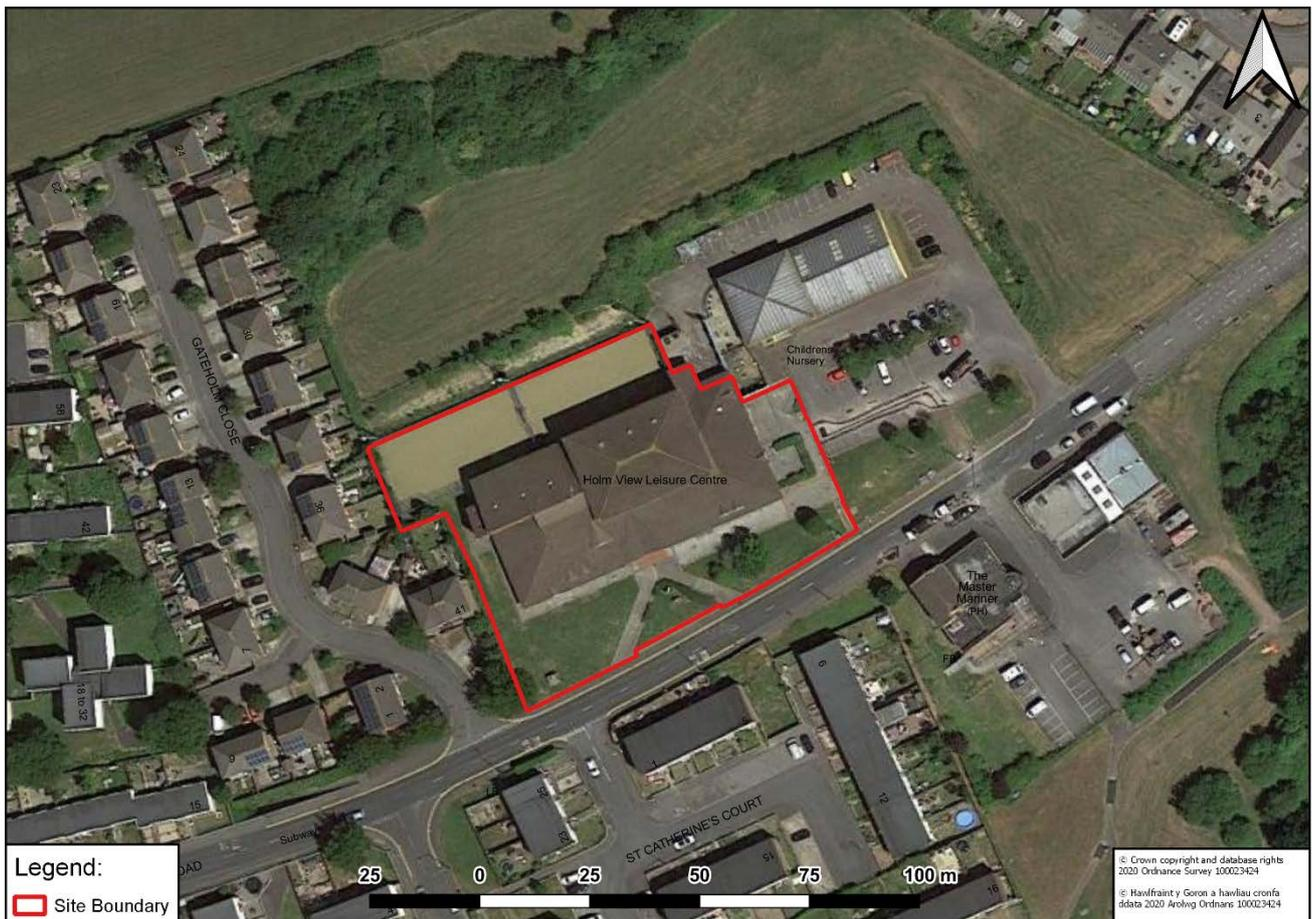
3.2. The Holm View Leisure Centre is a steel frame structure of pre-cast concrete slab construction with brickwork external cladding and a tradition pitched roof with a tiled roof. Built in Circa 1985, the building has an approximate internal area of 2,000 sq.m. The existing building has no particular architectural merit and consideration would be given to either the retention, conversion, extension or replacement of the existing building on the site.
