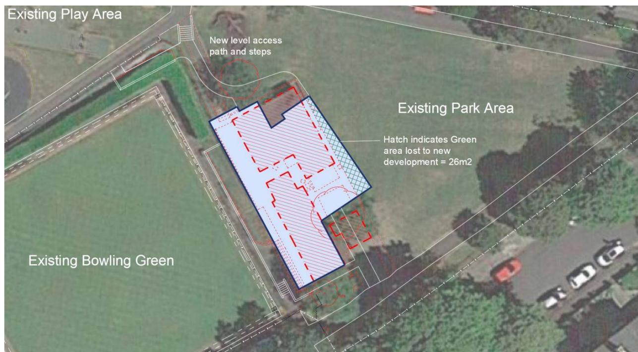
Figure 16: Hatched area indicates green space lost to the new development.
