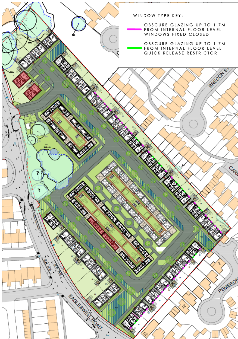
Fig 5: Layout plan indicating plots with obscure glazing/film and fixed windows or windows with quick release restrictors to rear elevations
